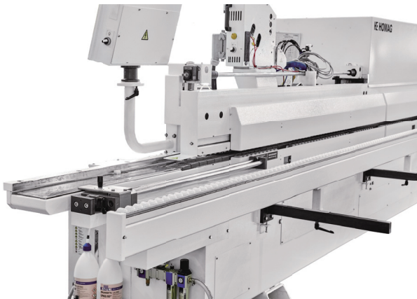
Infeed device: For narrow parts infeed in crosswise.
